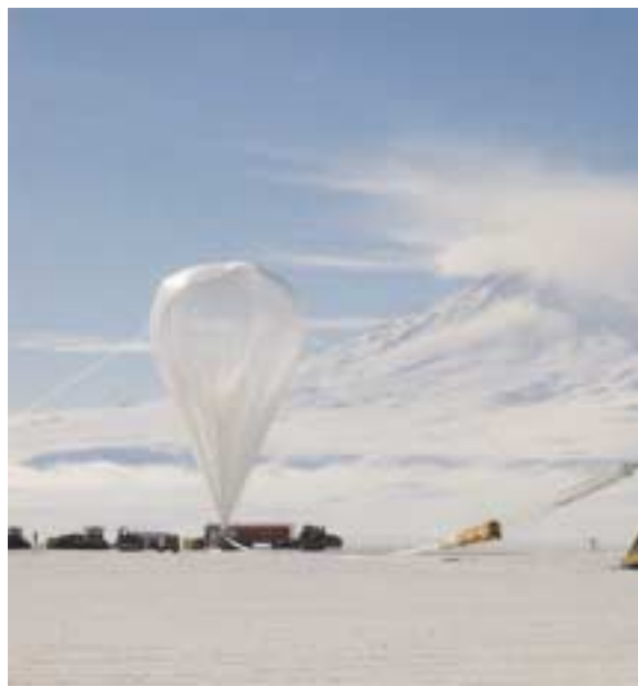
In late 1998, the BOOMERANG balloon telescope was launched to measure cosmic microwave background radiation. This balloon carried the telescope for 10 days while circumnavigating Antarctica. Image courtesy of NASA.
